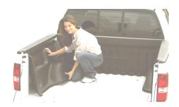
Align the holes in the sidewalls with the holes in the loadguard. You may use a Phillips screwdriver or punch as an alignment tool.
